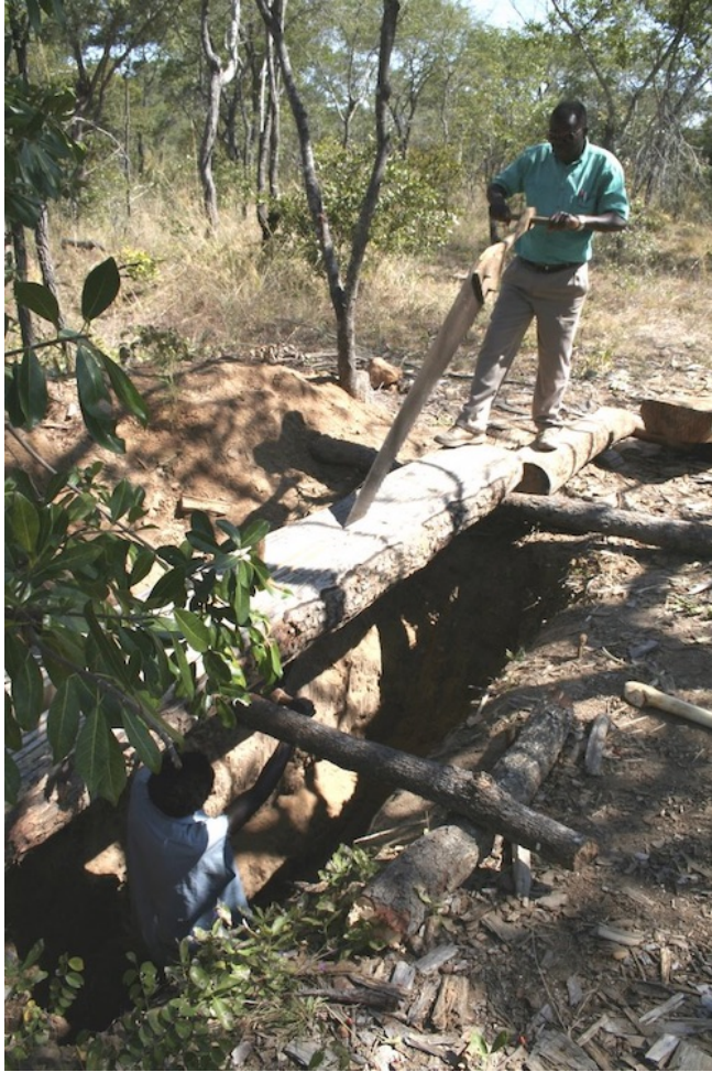
Figure 3 Two men use a pit saw in Kalomo town, Southern Province, Zambia. Photo by Amanit Phalloides - Namwianga Mission, CC BY-SA 3.0, https://commons.wikimedia.org/w/index.php?curid=1534654
